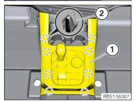
• Correctly position the centre console trim (1) and engage at the clamps (2).
