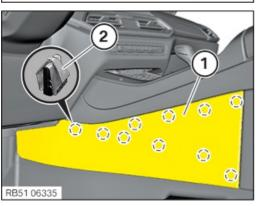
• Clip in the carpet at the side of the centre console (1) starting from the front at the clamps (2) and install.
